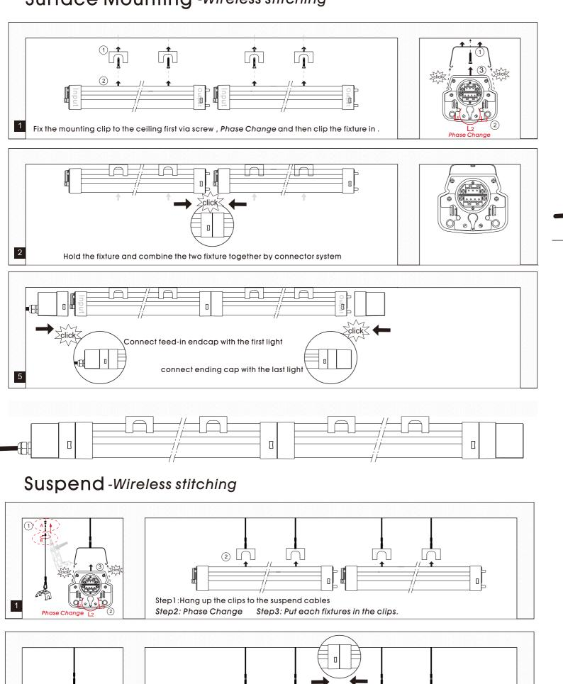
Hold the fixture and combine the two fixture together by connector system
